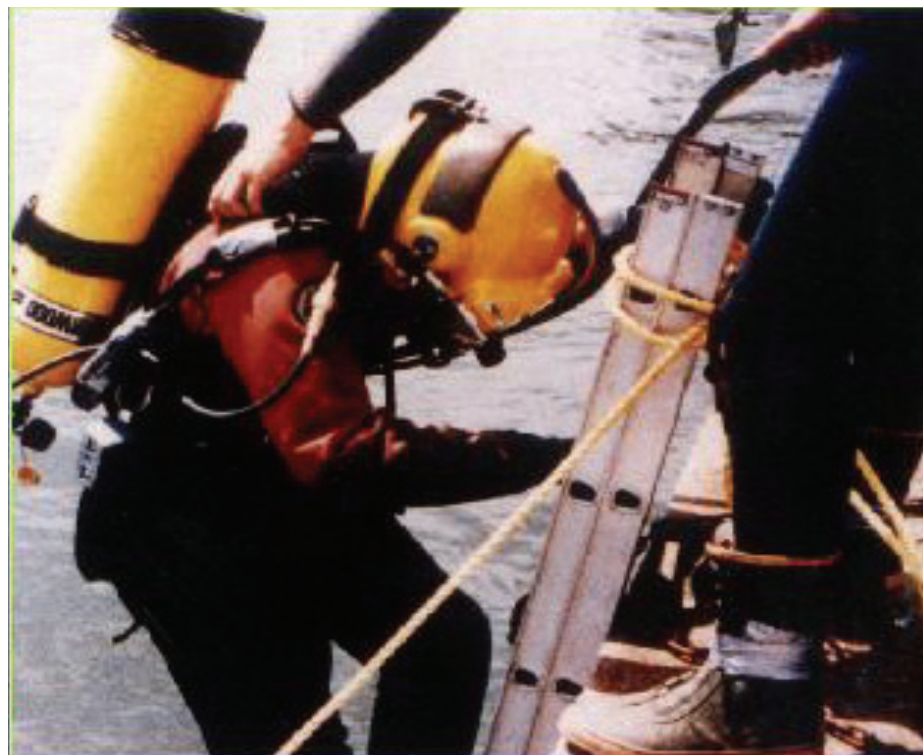
Figure 11.3.35 Surface-Supplied Diver with a Reserve Air Tank
