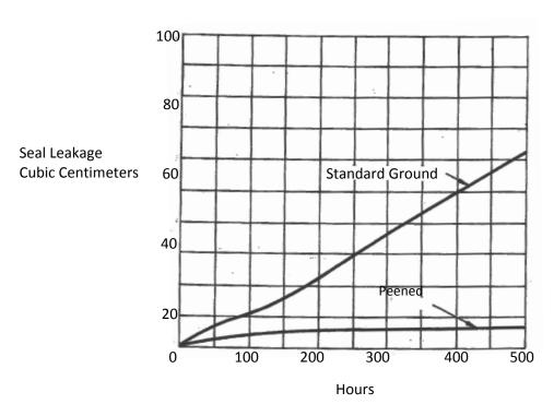
Shot peening isn't the only method by which the fatigue life of a part can be increased. Others include cold working by rolling, stretching, compressing, twisting; heat treating including induction hardening and flame treatment; and altering the surface composition by "carburizing", "nitriding", etc. However, shot peening possesses advantages over all of the above such as improved flexibility, control, safety and cost.
