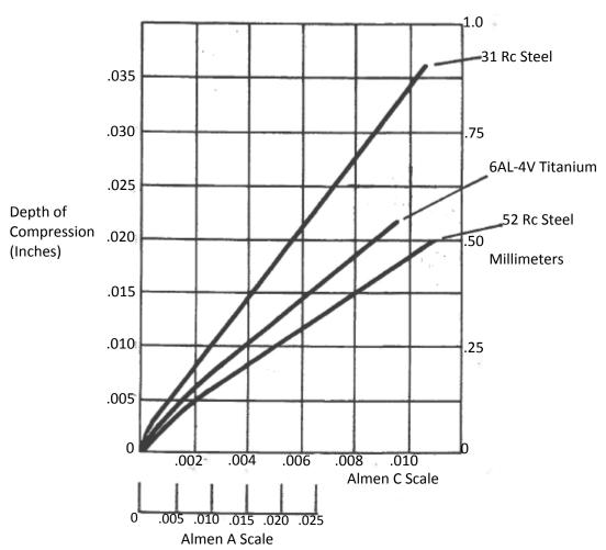
For parts having a thickness of 1/16 inch or less, a slurry of very small glass beads and water, propelled by pressurized air, has been found to create the best results. The results, similar to those using air-propelled dry metal shot, create small craters of cold worked material. Since the glass beads are smaller than metal shots, the craters are smaller, creating a very thin layer of compressed stress established in the work piece.
