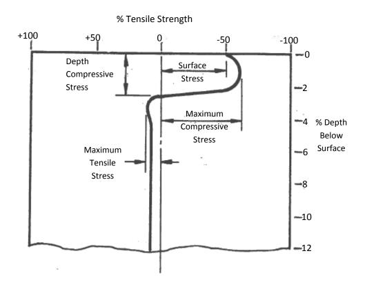
Figure 2 below has a graph demonstrating the magnitude of the induced compressive stress in shot peened steel. It plots induced compressive stress versus tensile strength of steel. It demonstrates the above-mentioned principle that the compressive stress induced by shot peening is at least one-half the tensile strength of the material being treated. Variations in the shot peening
