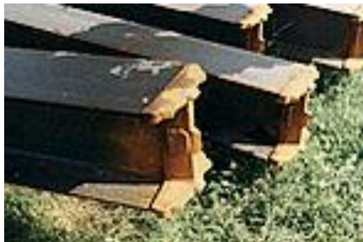
Figure 5 Example of pile tips.
