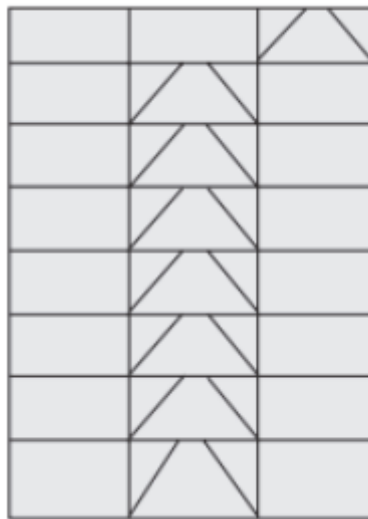
Figure 9. Example of an in-plane discontinuity irregularity
