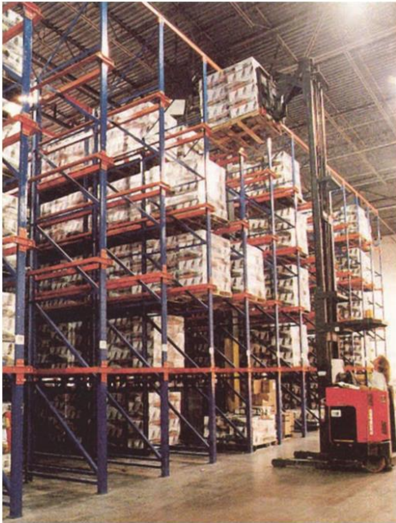
Figure 7. Seismic design criteria for steel storage racks of the type used in large warehouses and big-box retail stores are included in the building code.
