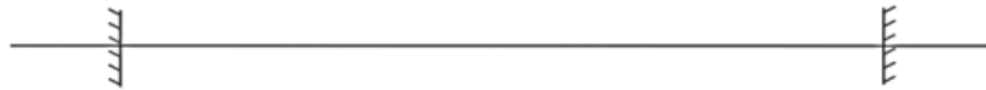
Figure 26. Analogy schematization of double leaf Bascule Bridge with active mid-span moment locks
