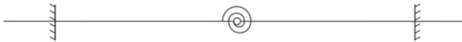
Figure 22. Schematization of real behavior double leaf Bascule Bridge with active mid-span shear locks
