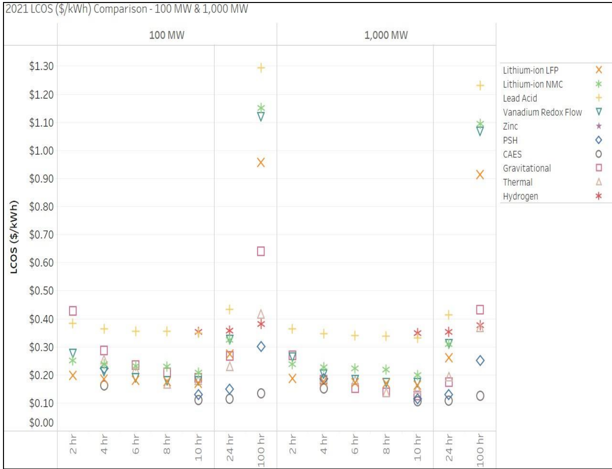
Figure 3. Comparison of LCOS ($/kWh) by Technology, Power Capacity, and Duration
