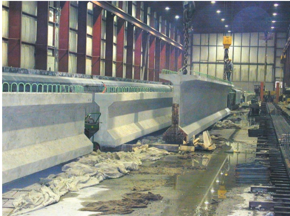
Figure 5.2.7 Prestressed Concrete Beams with Shear Connectors Protruding
