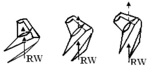
Figure 5-6 Effect of Elevator
