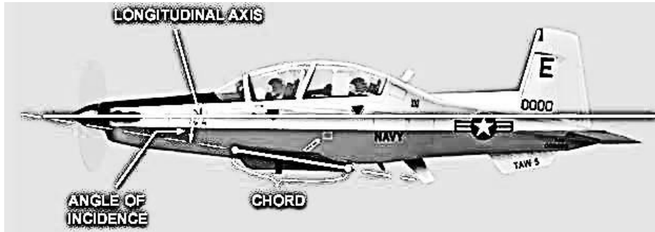
Figure 1-15 Angle of Incidence
