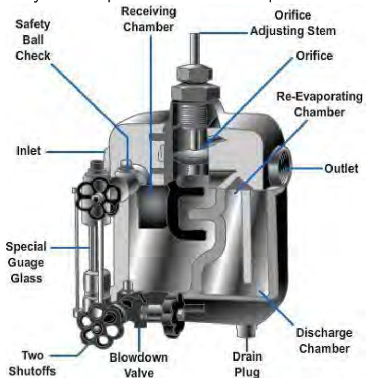
Figure 10-17 – Throttling trap.
