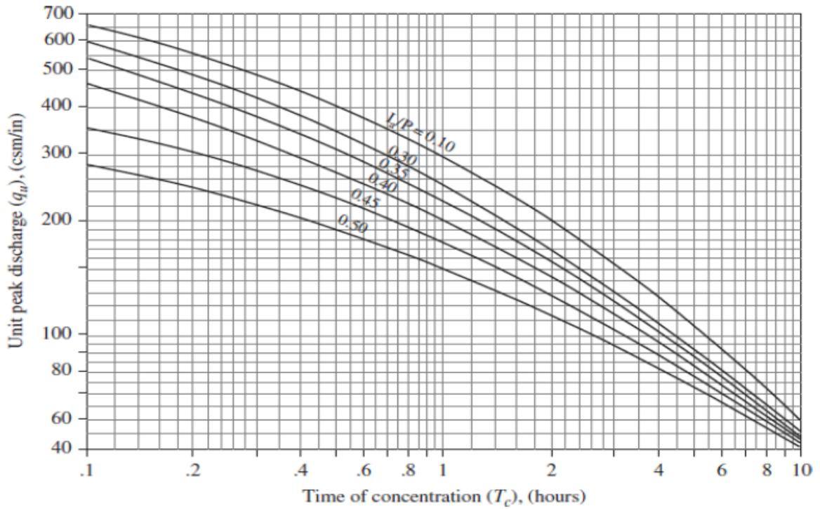
Figure 15 Unit Peak Discharge ( $q_u$ ) for Type III Rainfall Distribution (NRCS, 1986)
