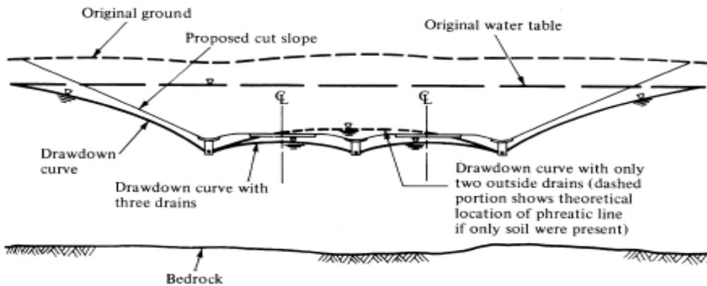
Figure 20 Multiple Longitudinal Drawdown Drain Installation
