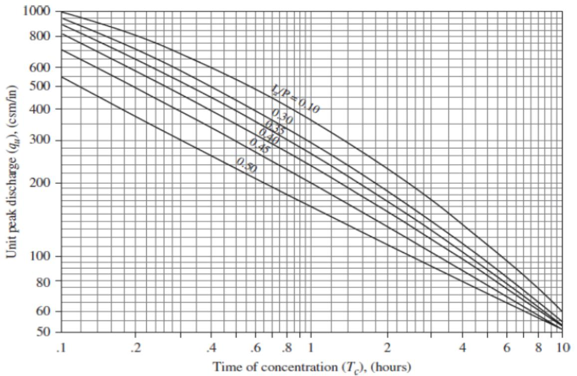
Figure 14 Unit Peak Discharge ( $q_u$ ) for Type II Rainfall Distribution (NRCS, 1986)
