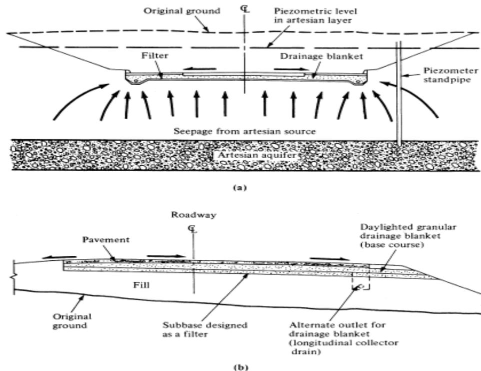
Figure 22 Applications of Horizontal Drainage Blankets
