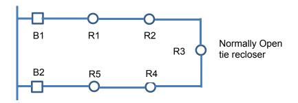
To make coordination easier, some reclosers can lower their tripping characteristics when they operate in reverse mode. So, in this particular case, recloser R2 would drop its current pickup setting. Recloser R2 sees lower fault currents than it normally does and it needs to open before reclosers R3 or R4. In the event a fault occurs between breaker B1 and recloser R1, the loop consisting of five reclosers will respond in a similar way it would respond in the case of the three-recloser loop:
